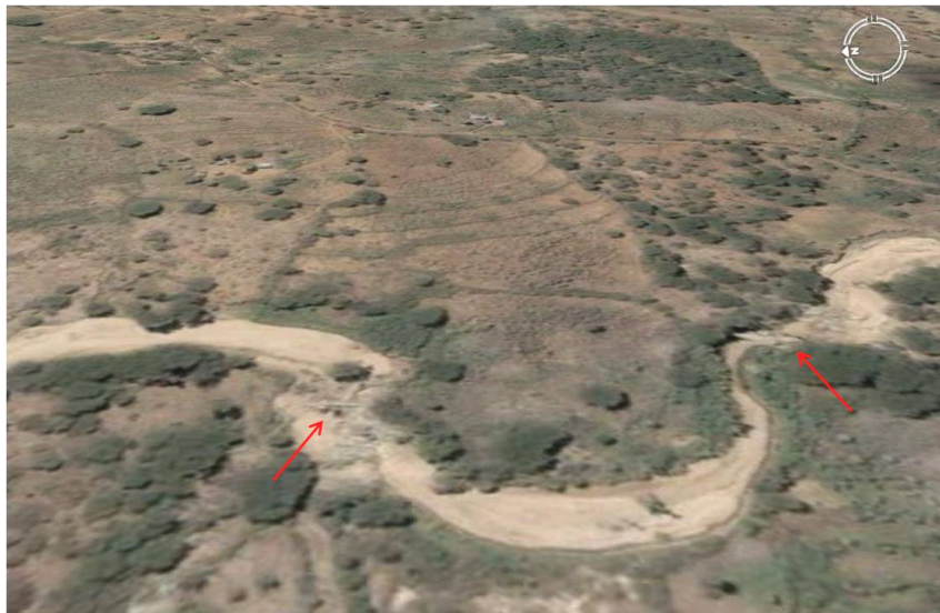
Figure 1.2 Two dams in an ephemeral river. The bright colour is accumulated sand (source of satellite image: Google Earth).
