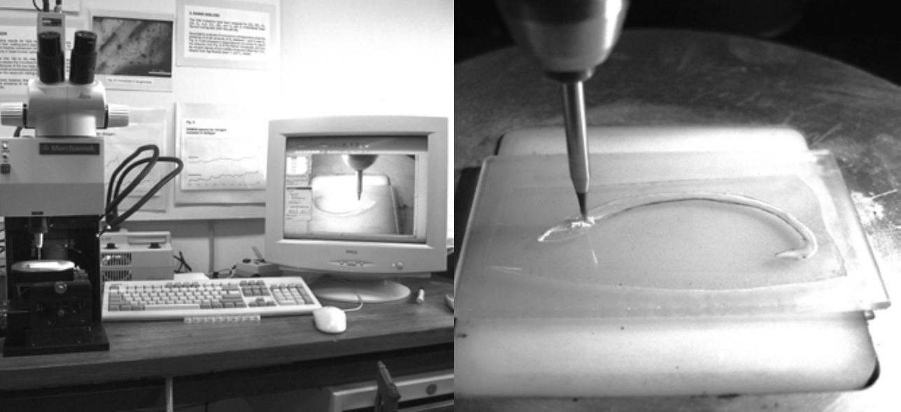
Figure 1.12a-b: The Merchantek Micromill drilling a shell sample. Samples are mounted on a computer-controlled XYZ-stage under a fixed dental drill. Software allows complex drill patterns to be drawn.
