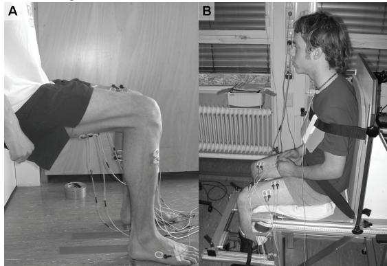
Figure 2.1 A) Set-up of Experiment 1: Participant is leaning against the wall in the 90^\circ condition. B) Set-up of Experiment 2. Participant is sitting in an adjustable chair with force sensors at shin level.
