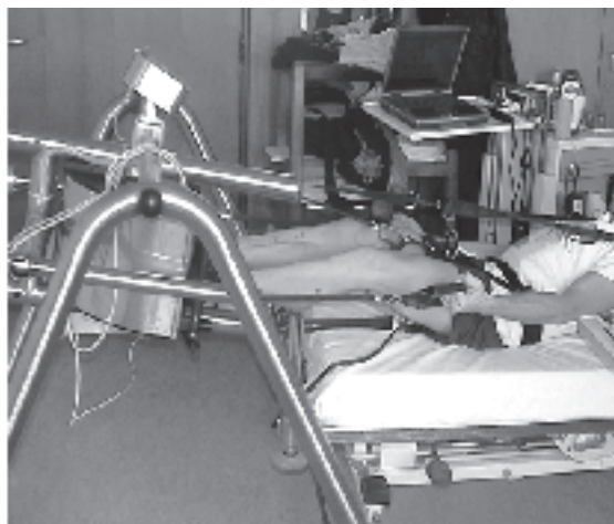
Fig. 1. The Galileo Space Device used for resistive vibration exercise at supine position during 56 days of strict bed rest.
