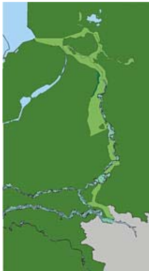
Figure 8.2 The proposed bypass and restructured IJssel river. The light grey areas are currently flood-safe, but will occasionally flood in the proposed situation. Source: Delft Hydraulics, 1998. See also Figure 6.2.
