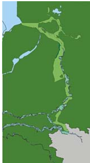
Figure 6.2 The proposed bypass (see also Figure 6.3) and restructured river IJssel. The light grey areas are currently flood-safe, but would occasionally flood in the proposed situation. Source: WL/Delft Hydraulics, 1998.
