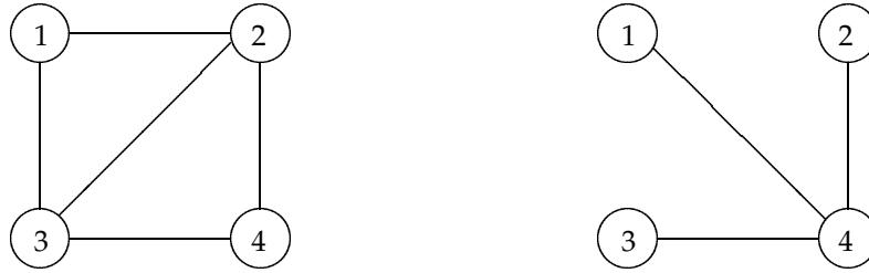
Figure 3.3: The two offspring obtained by an application of one-point crossover to the individuals of example 3.1.
