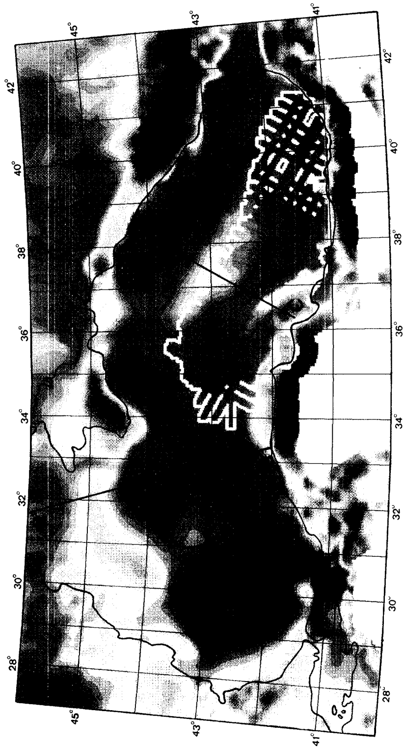
Fig. 2. Free-air gravity map of the Black Sea and location of the profiles analysed by our gravity modelling procedure (Figs. 3 and 4). Colours indicate values from 230 mGal (bright pink) to -100 mGal (dark blue). See also Figs. 3 and 4 for free-air gravity anomaly values along the modelled profiles.
