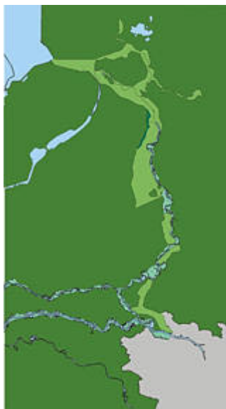
Figure 4.1 The proposed bypass and restructured IJssel river. The light green areas are currently flood-safe, but will occasionally flood in the proposed situation. Source: Delft Hydraulics (1998).
