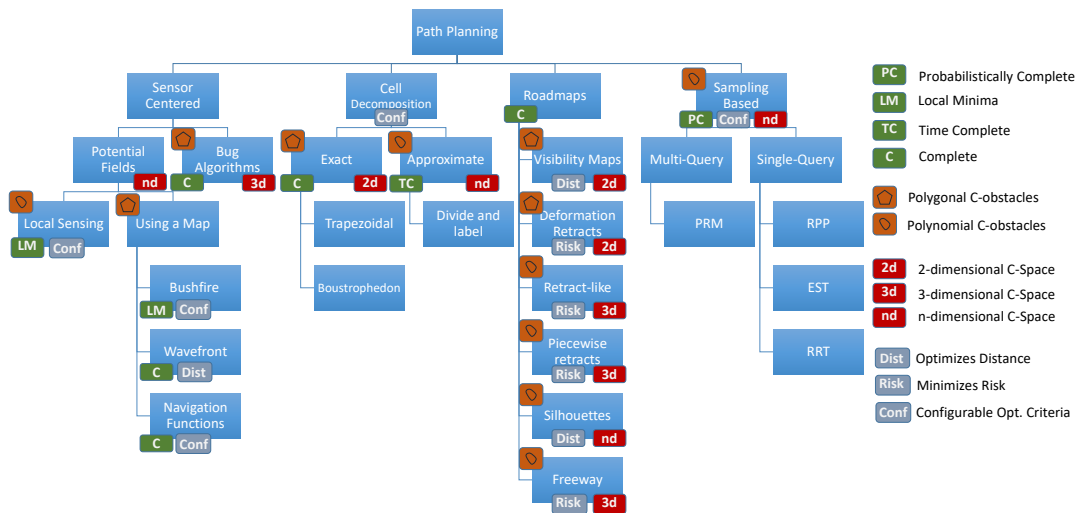
Figure 2.2: Path planning algorithms. Their classification for completeness (green), c-obstacle complexity (orange), c-space dimensionality (red) and optimization criteria (blue) are shown.
