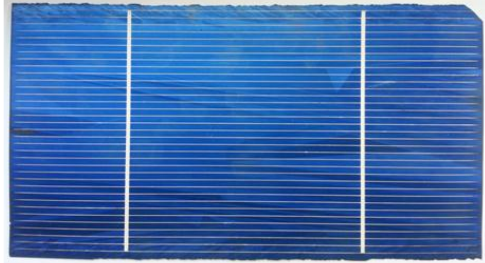
Figure 18. Ribbon growth (EFG) Si solar cell.
