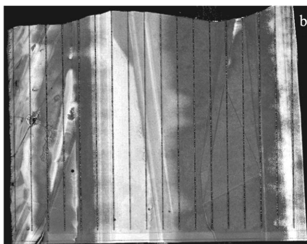
Figure 54. SAM of polycrystalline sample 2 (a) before and (b) after cracking.
