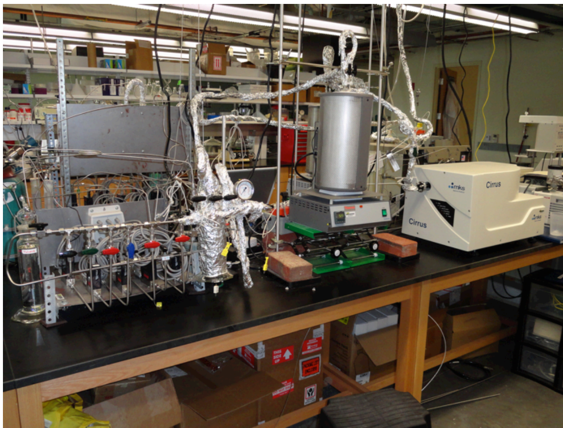
Figure 5: Reactor used in tri-reforming experiments.
