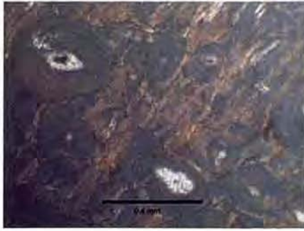
Fig. 2 Area of bone with well-preserved osteons, as observed via optical microscopy.
