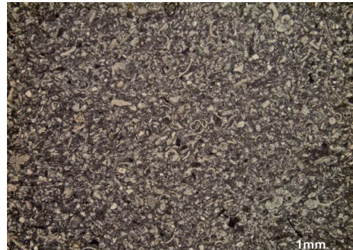
Fig. 7. Photomicrograph of the sample E25 (X1618). Very slightly sandy, compact bioclastic packstone – Platja de Binigaus, cliff.
