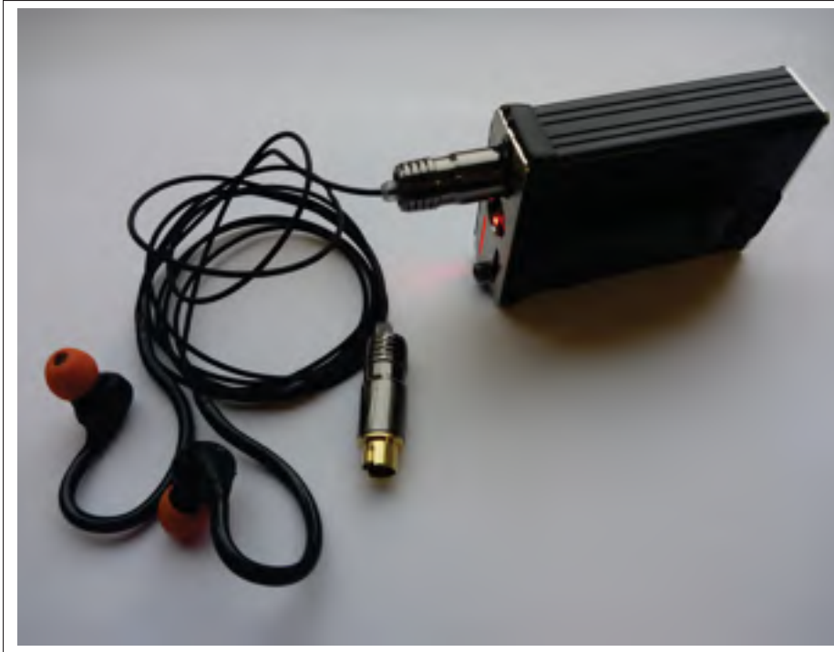
Figure 4.6 The auditory research platform in which the speech enhancement algorithm is implemented for real-time processing connected to two earpieces for enhanced signals transmission.
