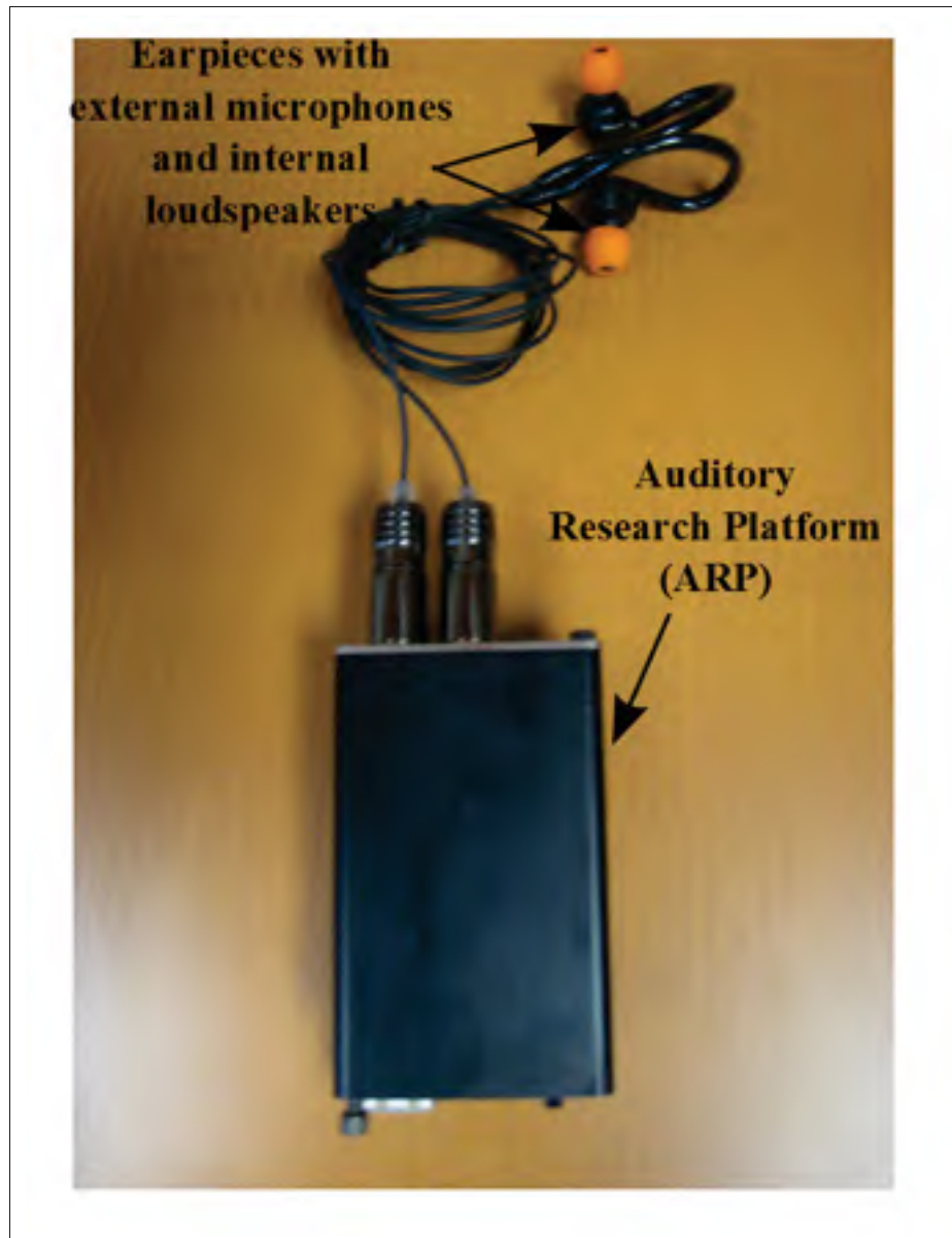
Figure 3.8 The auditory research platform in which the VAD is implemented for real-time processing connected to two earpieces for audio signal acquisition and VAD's decision transmission.
