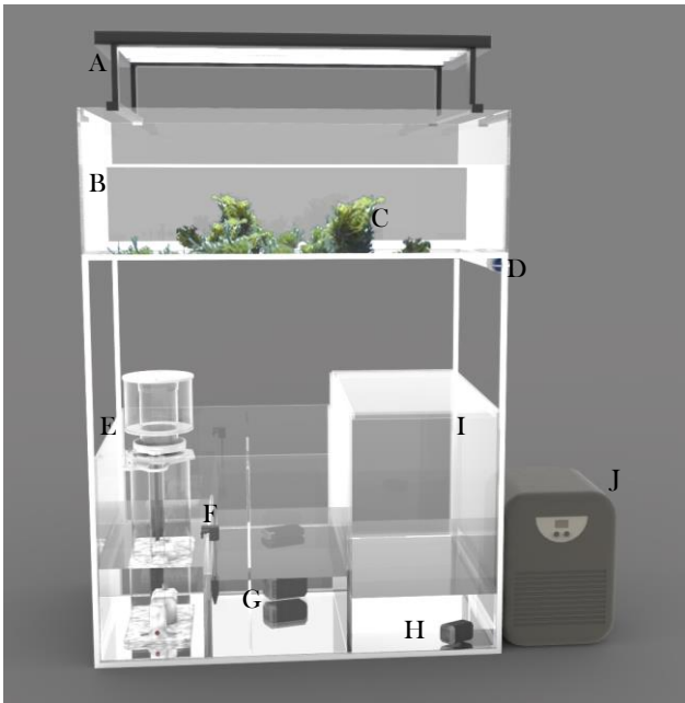
Figure 3. Schematic drawing of the Life Support System in which the studies described were conducted. The items used are: A - Lights; B - Aquarium where the trays were placed; C - Illustration of Codium tomentosum ; D - UV light; E - Protein skimmer; F - Level measurer; G and H - Water pumps; I - Osmose water reservoir; J - Refrigerator.
