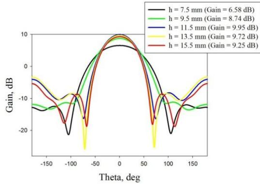
Figure 3. Gain at various height of the RDR
