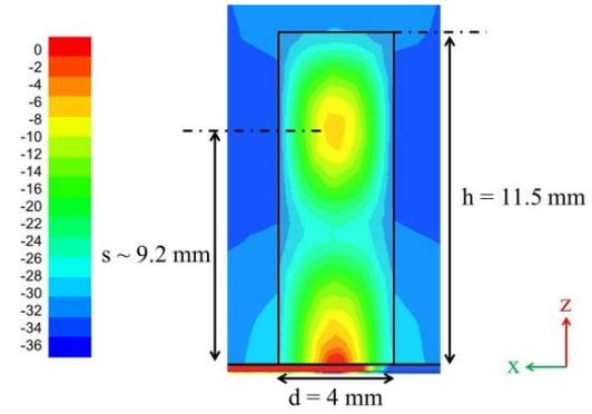
Figure 4.  $H_y$  field in  $TE^y_{1\delta 3}$  mode
