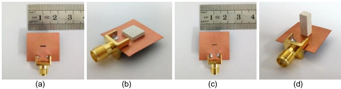
Figure 9: Photograph of the fabricated RDRA (a) Top view without RDR in the  $TE^y_{1\delta 1}$  mode (b) 3D view with RDR in the  $TE^y_{1\delta 1}$  mode (c) Top view without RDR in the  $TE^y_{1\delta 3}$  mode (d) 3D view with RDR in the  $TE^y_{1\delta 3}$  mode
