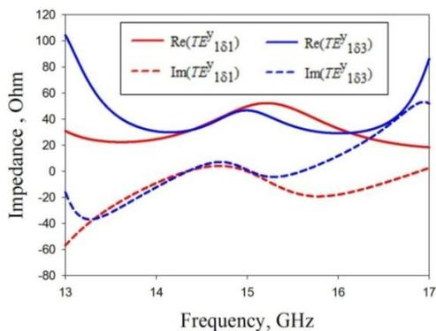
Figure 10. Comparison of the impedance matching
