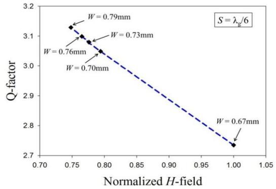
Figure 8. Loaded  $Q$ -factor influenced by coupling mechanism
