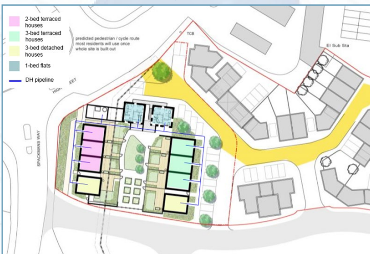
Figure 7-2 Layout of the district heating network.
