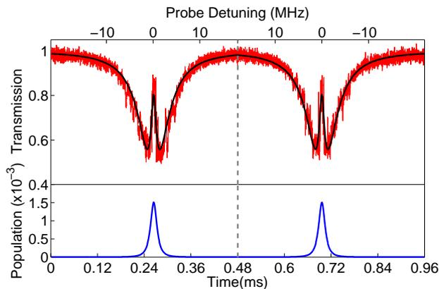
**Figure 4.** (Color online) Top: Double scan EIT for the  $|1\rangle \rightarrow |2\rangle \rightarrow |3\rangle = 26d$  system with a probe power of 200 nW and coupling beam power of 60 mW. The solid line (black) is the theoretical line of best fit giving an EIT linewidth of  $0.58 \pm 0.04$  MHz. Bottom: Population of the Rydberg state as a function of time for the duration of the scan.
