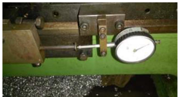
Fig.16 Dial indicator for accurate movemet of the movble cutter for acurate results
