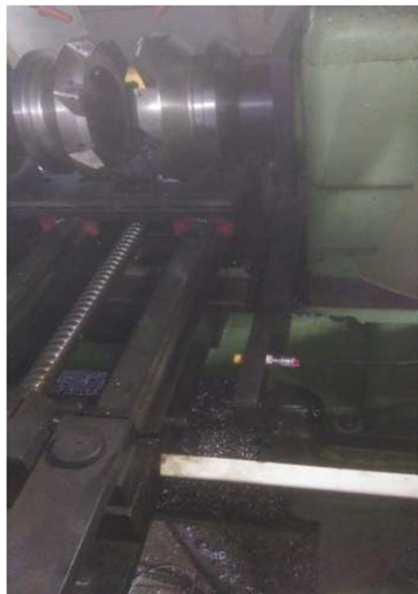
Fig. 27 Motion of bed back to home from proximity sensor 2
