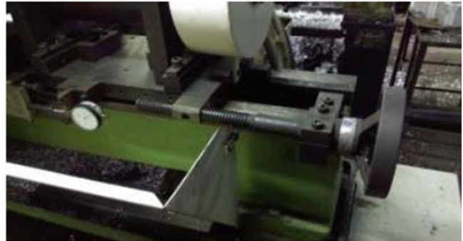
Fig.14 Forward reverser motion of movable cutter with the help of handle
