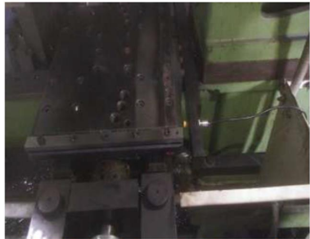
Fig. 26 Bed reached at the Proximity sensor 2
