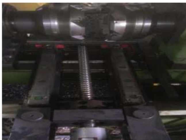
Fig. 22 Ball Screw connected to servo motor for T o and FRO motion of bed
