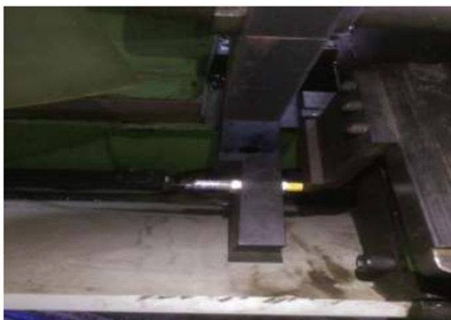
Fig. 17 Checking the position of bed at home by proximity sensor 1
