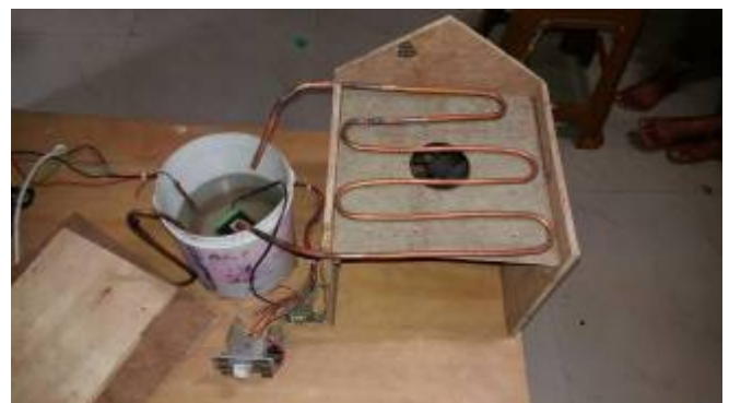
Fig 8: radiant cooling coil arrangement
