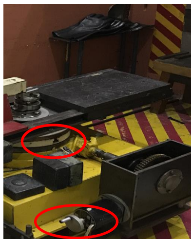
Figure 3: Rotatory adjustment with the function of aligning the spectrometer to the irradiation beam of J-9 channel.
