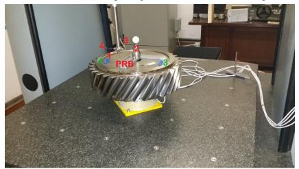
The calibration was carried out in two steps, following common practice at INRIM for calibrations by means of coordinate metrology.
