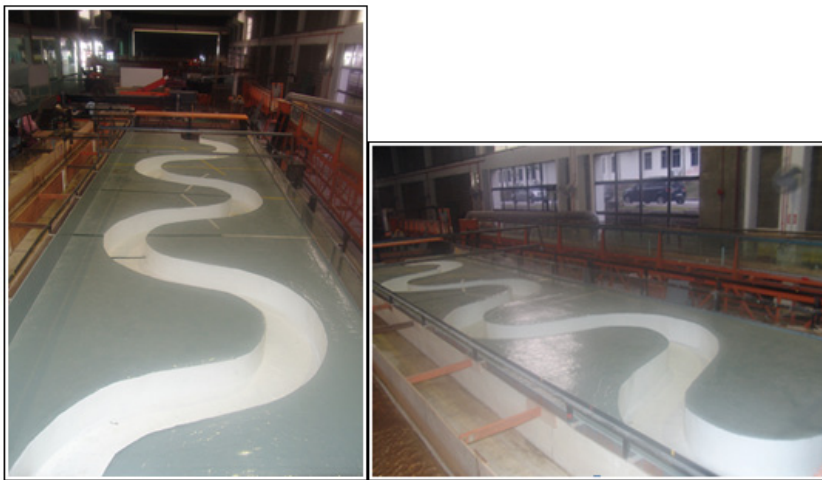
Fig.3: Laboratory meandering flume at UTM
