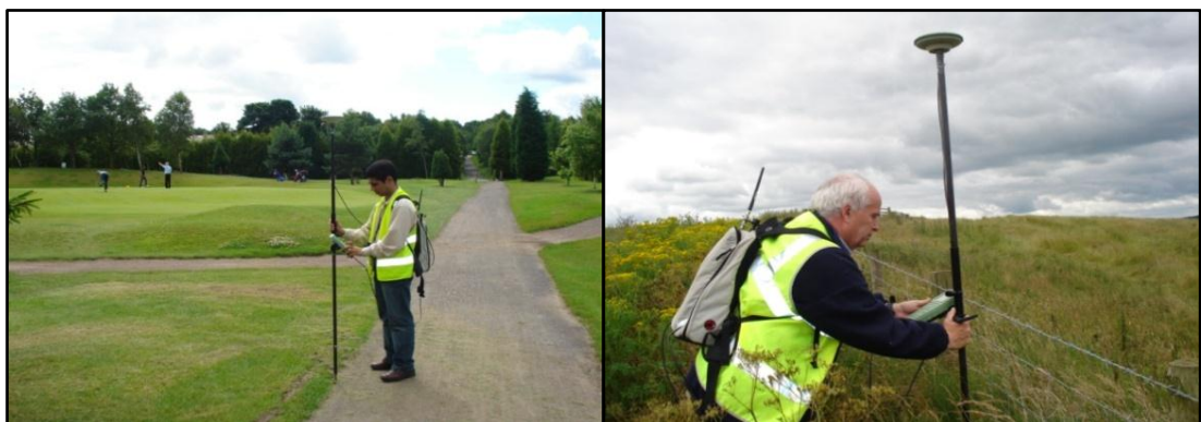
Figure 4.5 GPS Leica GX1230, employed to survey the location of features in open-space area using RTK technique
