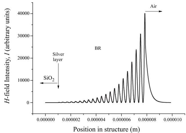
FIG. 5. The time-averaged  $H$ -field intensity associated with the 1.32 eV interface state. The region considered is composed of 1000 nm of  $\text{SiO}_2$  substrate, 57 nm of silver, 20 pairs of  $\text{SiO}_2/\text{TiO}_2$  layers giving a 6833 nm wide BR with a 2000 nm region of air on the right.
