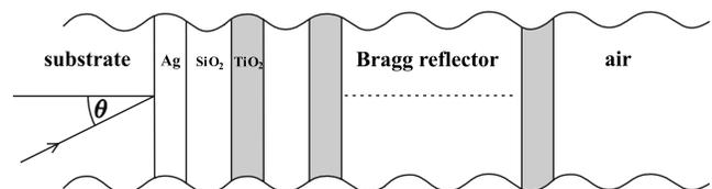
FIG. 1. The basic structure employed in most of the calculations, consisting of a left-hand substrate (SiO<sub>2</sub> in this case) with a thin silver (Ag) overlayer and a 40-layer SiO<sub>2</sub>/TiO<sub>2</sub> BR (20 layer pairs) on top. For the reflection coefficient calculations light is incident at an angle  $\theta$  from the left.
