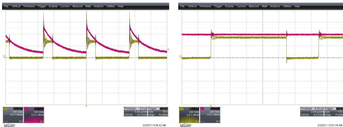
Figure 7: V DS (Yellow) V TOS (Red) (left); V DS (Yellow) V OVS (Red) (right)
