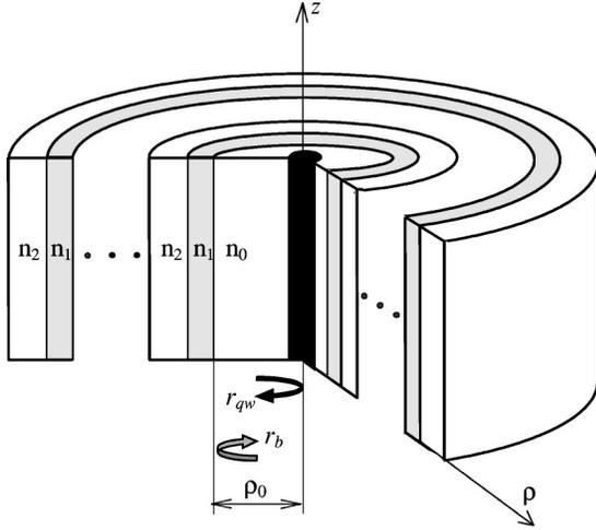
FIG. 1. An illustration of a cylindrical microcavity with quantum wire at its center. A central core of the refractive index  $n_0$  is surrounded by a cylindrical Bragg reflector, constructed from alternate layers of the refractive index  $n_1$  and  $n_2$ .
