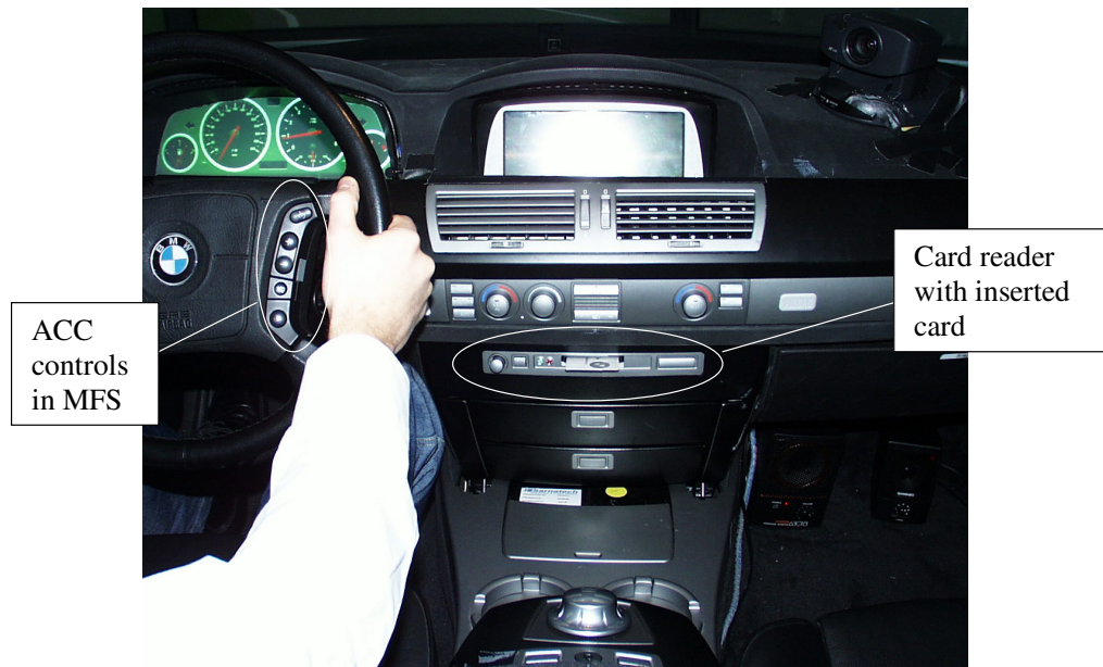
Figure 28. Implemented card reader in driving simulator cockpit and ACC buttons in MFS
