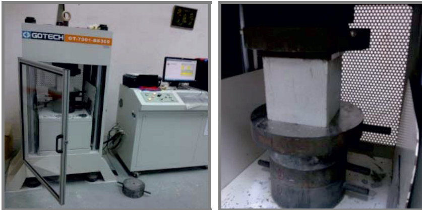
Figure 3. GOTECH GT-7001-BS300, with a 300ton-capacity compression machine.
