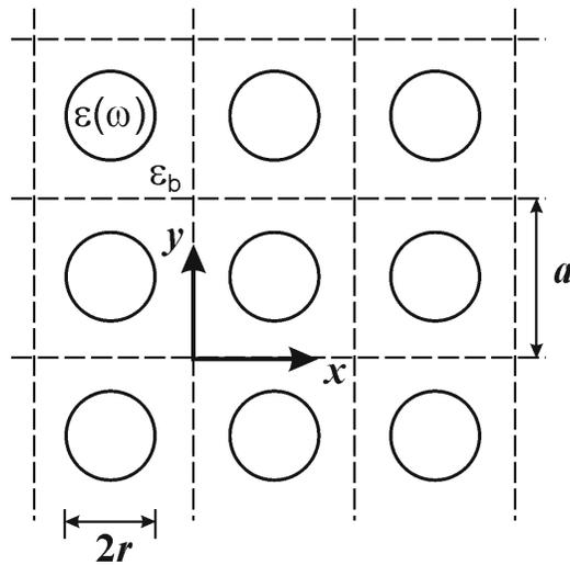
Fig.1 An array of circular rods having a frequency-dependent relative permittivity  $\varepsilon(\omega)$  embedded in a background material for which the relative permittivity has a constant value  $\varepsilon_b$ .
