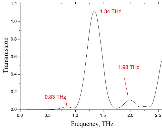
Fig. 3 Plot showing the transmission for a finite structure consisting of 6 layers of 50  $\mu\text{m}$  diameter gold rods in a 200  $\mu\text{m}$  lattice constant array. The FDTD approach is employed to calculate the transmission.
