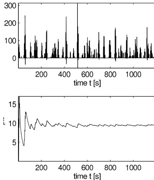
**Figure 8:** *The power in the power take off system is calculated using the solutions of velocity and force in an irregular wave regime. The top graph shows the power as a function of time. The bottom graph shows the power as a running average function over time. Power is measured in Kilowatts [kW].*
