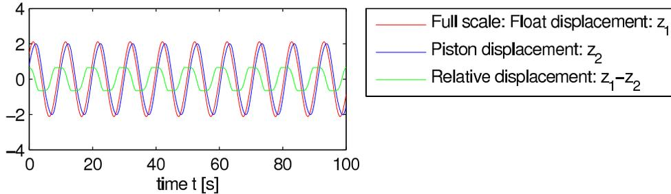
**Figure 3:** *Solutions of displacement in a regular wave regime. Displacement is measured in meters [m].*
