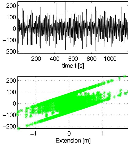
**Figure 7:** *The force in the power take off system is calculated using the solutions of displacement in an irregular wave regime. The top graph shows the force as a function of time. The bottom graph shows the force as a function of extension. Force is measured in Kilonewtons [kN].*
