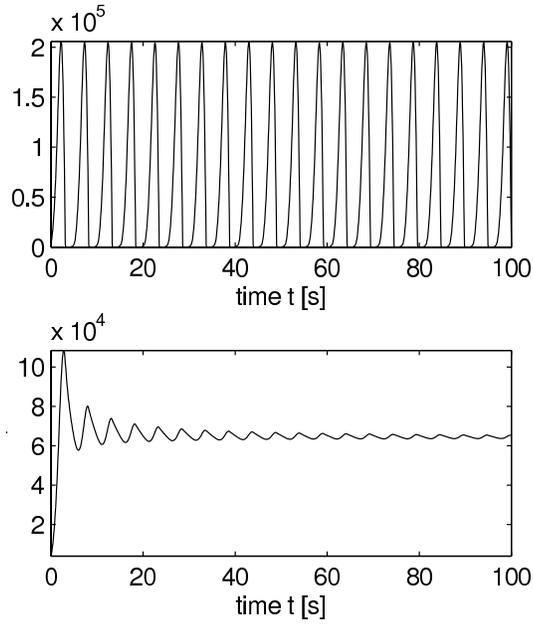
**Figure 5:** *The power in the power take off system is calculated using the solutions of velocity and force in a regular wave regime. The top graph shows the power as a function of time. The bottom graph shows the power as a running average function over time. Power is measured in Watts [W].*
