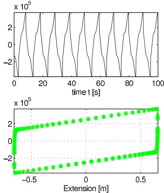
**Figure 4:** *The force in the power take off system is calculated using the solutions of displacement in a regular wave regime. The top graph shows the force as a function of time. The bottom graph shows the force as a function of extension. Force is measured in Newtons [N].*
