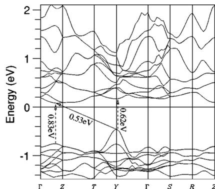
FIG. 5. The band structure of type-B  $\beta$ -FeSi<sub>2</sub> is shown here. The arrows indicate the smallest direct and indirect band gaps.
