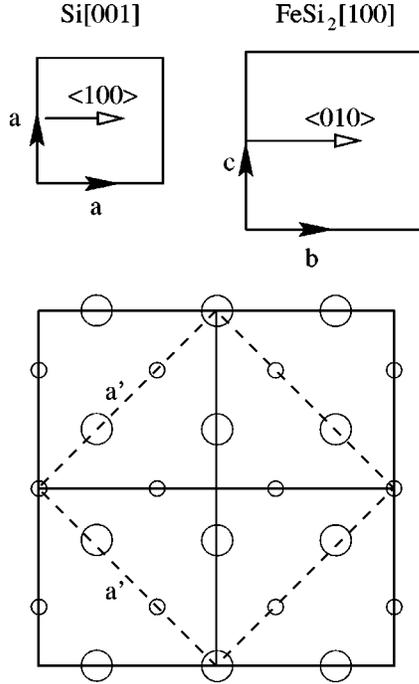
FIG. 2. Illustration of the type-B ( $\beta$ -FeSi<sub>2</sub>[010]||Si(001)) interface. The  $2 \times 2$  conventional  $\beta$ -FeSi<sub>2</sub>(100) surface cells are shown as full lines on top of the open circles indicating the top layer of atoms in the Si substrate. The lattice parameters  $b'$  and  $c'$  of the  $\beta$ -FeSi<sub>2</sub>(100) common unit mesh are given by  $b' = (0, 1, 1)b$  and  $c' = (0, -1, 1)c$ .
