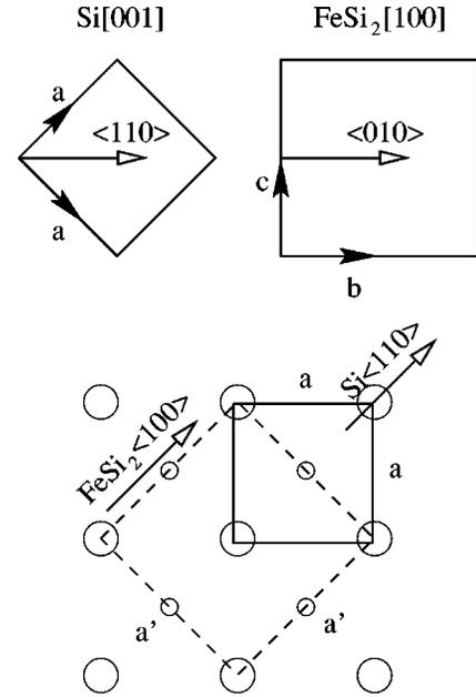
FIG. 1. The type-A ( $\beta$ -FeSi<sub>2</sub>[010]||Si⟨110⟩) heteroepitaxial relationship. The top diagram shows plan views of the conventional Bravais lattices of Si and  $\beta$ -FeSi<sub>2</sub>. In the bottom diagram the top layer of atoms in the Si cell are shown as open circles and a  $\beta$ -FeSi<sub>2</sub> cell (dashed lines) is chosen to coincide with the Si conventional cell, given a  $\pi/4$  rotation around the direction perpendicular to the substrate.
