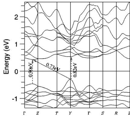
FIG. 4. The band structure of the fully relaxed bulk structure of  $\beta$ -FeSi<sub>2</sub> is shown along several lines of high symmetry. Arrows indicate the lowest-energy electronic band gaps. It can be seen (solid arrow) that the smallest band gap in this case is indirect between the Y point and the Z $\Gamma$  line.
