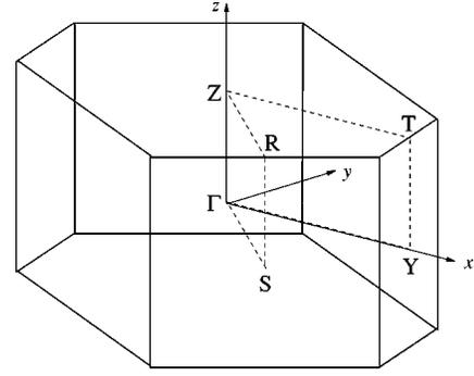
FIG. 3. Here we show the Brillouin zone of the the  $\beta$ -FeSi<sub>2</sub> structure (from the primitive unit cell) showing the lines along which the band structures shown in later figures were calculated.
