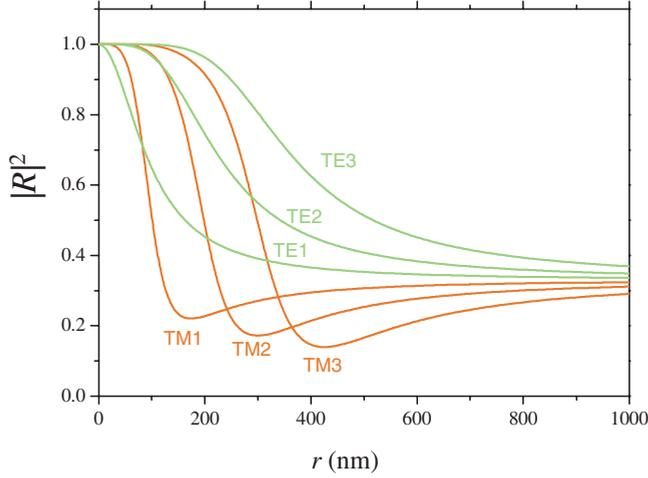
FIG. 1. (Color online) Power reflection coefficients of TE and TM outgoing spherical waves with  $l=1, 2,$  and  $3$  incident on a spherical interface of radius  $r$ . The refractive indices of the sphere and the surrounding medium are  $3.7$  (appropriate to GaAs) and  $1.0$ , respectively.
