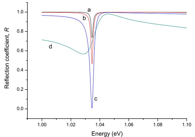
FIG. 4. (Color online) The TM reflection coefficient,  $R$ , at an angle of incidence of  $72.47^\circ$  for the structure with a 50 nm metal overlayer as a function of collision frequency: (a)  $\omega_c = 0$  rad s $^{-1}$ ; (b)  $\omega_c = 1 \times 10^{12}$  rad s $^{-1}$ ; (c)  $\omega_c = 1 \times 10^{13}$  rad s $^{-1}$ ; (d)  $\omega_c = 1 \times 10^{14}$  rad s $^{-1}$ .
