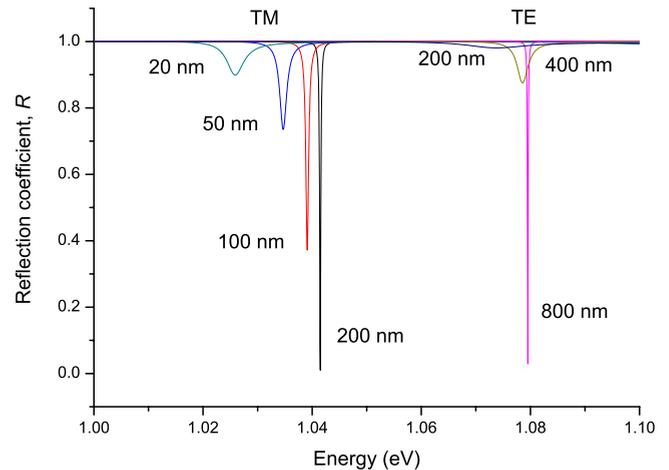
FIG. 3. (Color online) The TM and TE reflection coefficients,  $R$ , for a set of structures with different metal overlayer thicknesses (as labeled) on a 20-period AlAs/GaAs Bragg reflector on a GaAs substrate. Light is incident from the left, in air, at an angle of  $72.47^\circ$  to the normal for the TM polarization and  $67.06^\circ$  for the TE polarization.
