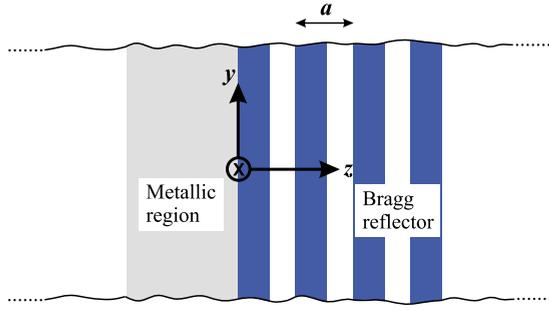
FIG. 1. (Color online) Schematic diagram of the structure, comprising a semi-infinite metallic region on the left and a semi-infinite Bragg stack structure on the right with their interface at  $z=0$ . The shaded layers on the right correspond to the lower refractive index regions. The period of the Bragg reflector is  $a$ .
