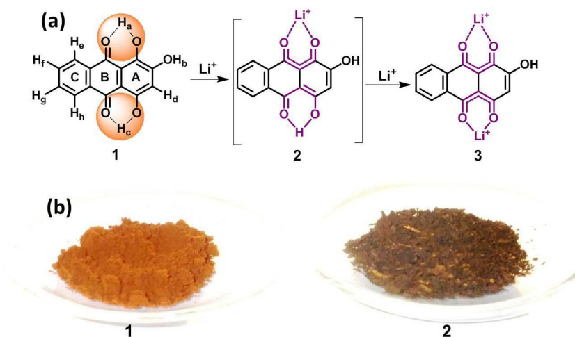
Figure 2 | (a) Schematic illustration of sequence of lithiation/de-lithiation mechanism in the purpurin molecule: (1) Molecular structure of pristine purpurin; (2) Intermediate of lithiated purpurin, and (3) Binding of lithium ion with carbonyl and hydroxyl groups of purpurin at C-1 ( -\text{OH}_a ) and C-4 ( -\text{OH}_c ) respectively. (b) Photograph of (1) pristine purpurin and (2) Chemically lithiated purpurin (1 : 2 ratio).
