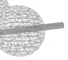
the field are not visible when rendered since they only serve to generate the mesh. By duplicating the elements, one can add them back in visually so that the position of the elements is understood when studying how the mesh reacts to the position of the individual elements.
