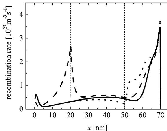
FIG. 5. Recombination rate in the active layer for a device with  $z=0$  nm (solid line) and  $z=20$  nm in Cases I (dashed line) and II (dotted line). Vertical dashed lines indicate the boundary of the low-mobility layer for the Case I (left) and Case II (right) devices.
