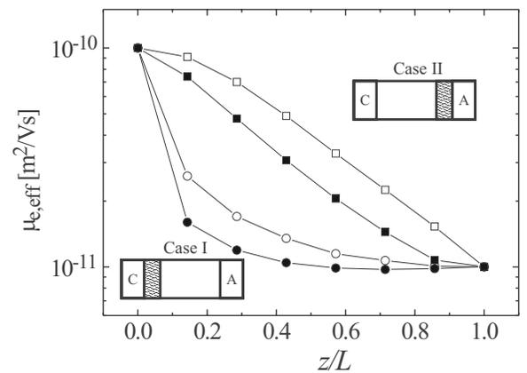
FIG. 2. Simulated (open symbols) and analytical (closed symbols) results for the effective electron mobility as a function of the fraction of the device comprising the lower mobility,  $z/L$ . Case I and Case II are represented by circles and squares, respectively. The insets illustrate the position of the region with low electron mobility (shaded area) relative to the cathode (C) and anode (A). Lines are a guide to the eye.
