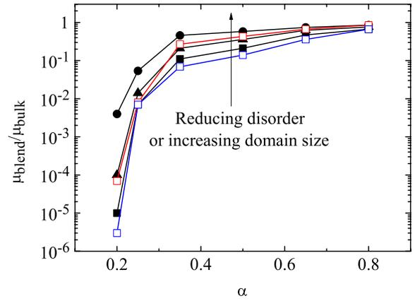
FIG. 1. (Color online) The ratio of electron mobility in the blend  $\mu_{\text{blend}}$  to that in the bulk  $\mu_{\text{bulk}}$  as a function of volume fraction of the acceptor material to the total volume  $\alpha$ . Squares, triangles, and circles represent blends with  $d=4, 8,$  and  $12$  nm, respectively. Energetic disorder is either  $\sigma=0$  (red),  $100$  meV (black), or  $125$  meV (blue). Lines are a guide to the eye.
