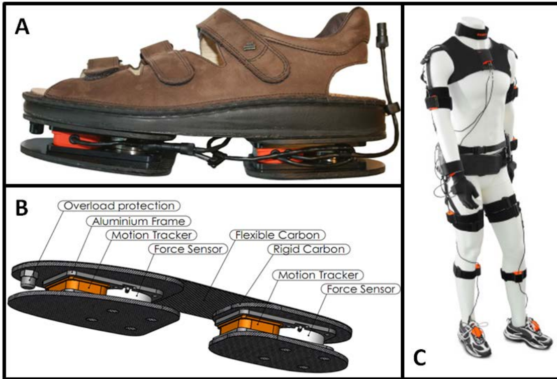
121 Fig. 2. Overview of the ambulatory measurement system used in the present study (Xsens technologies B.V., Enschede). (A) 122 Picture of one of the instrumented force shoes (FSs). (B) 3D representation of the force/torque and IMU sensors, and 123 mounting plates underneath each FS. (C) Full-body inertial motion capture (IMC) system.
