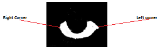
Figure 4.8: Sclera length estimation technique adopted by calculating the two corners from the segmented mask [275].
