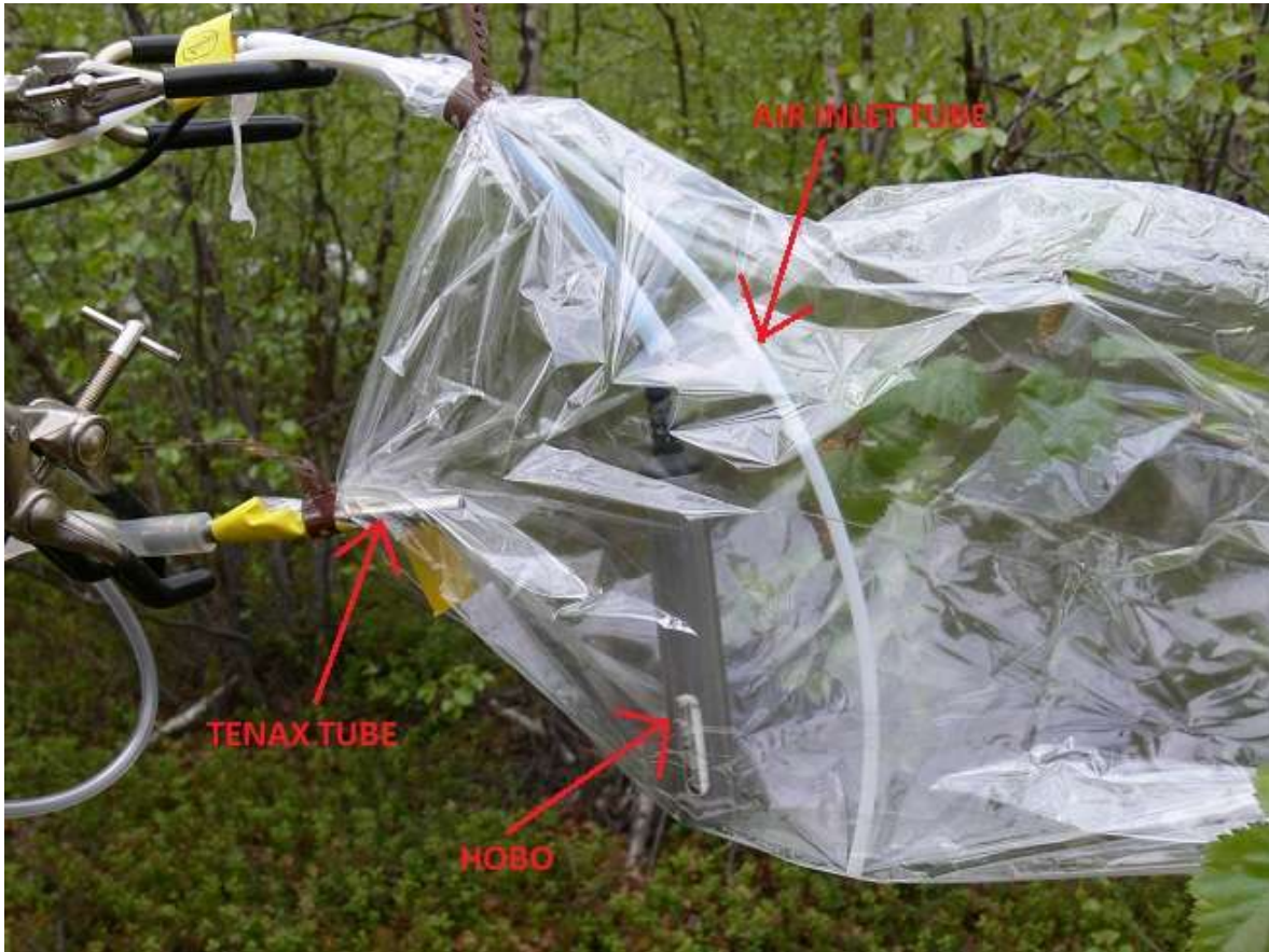
Picture 3. The sampling bag with HOBO, air inlet tube and Tenax tube with intake tube (Original Picture: Panu Piirtola 2007)
