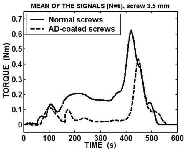
**Figure 7.2:** Mean insertion torque ( $N = 6$ ) of DLC-coated (AD-coated) and non-coated screws of diameter 3.5 mm in human bone.
