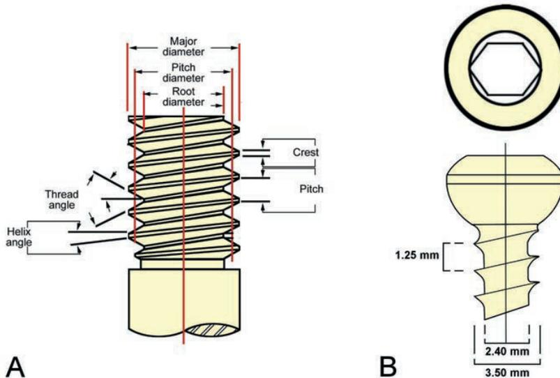
**Figure 3.1:** A) Screw anatomy with definitions. B) Dimensions of cortical bone screw used in the present study. (Modified from [53].)
