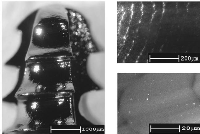
**Figure 6.1:** A tip of a DLC-coated self-tapping bone screw is shown on the left (screw diameter 3.5 mm). The inserts show optical micrograph (upper) and SEM (lower) of the screw with different magnifications.
