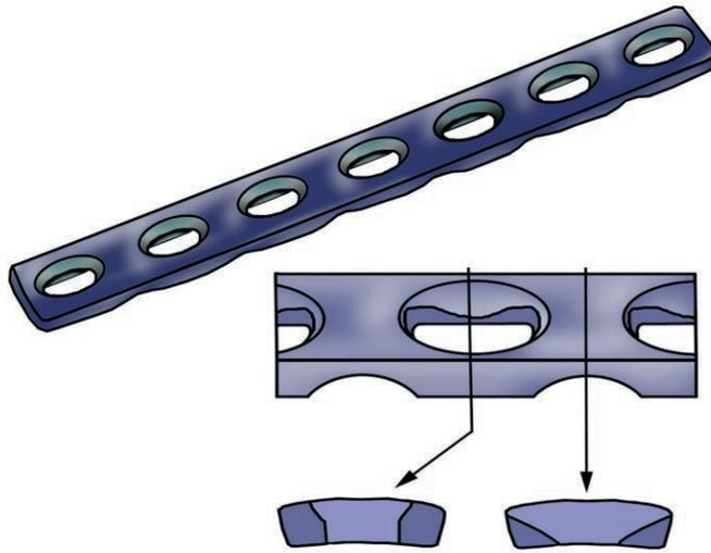
**Figure 3.3:** A design of a fixation plate used together with fixation screws in plate fixation. (Modified from [53].)
