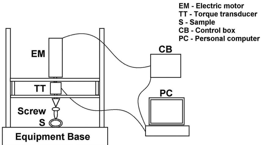
**Figure 6.3:** Schematic illustration of the developed test equipment for torque measurements.
