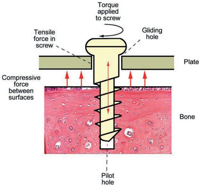
**Figure 3.2:** Mechanism of conventional plate fixation by generating compression between the plate and the bone for stability. (Modified from [53].)
