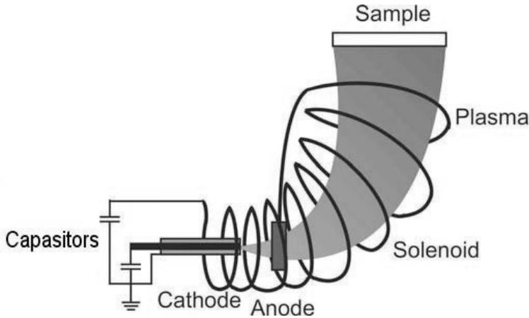
Figure 4.3: Schematic illustration of the FPAD coating system.
