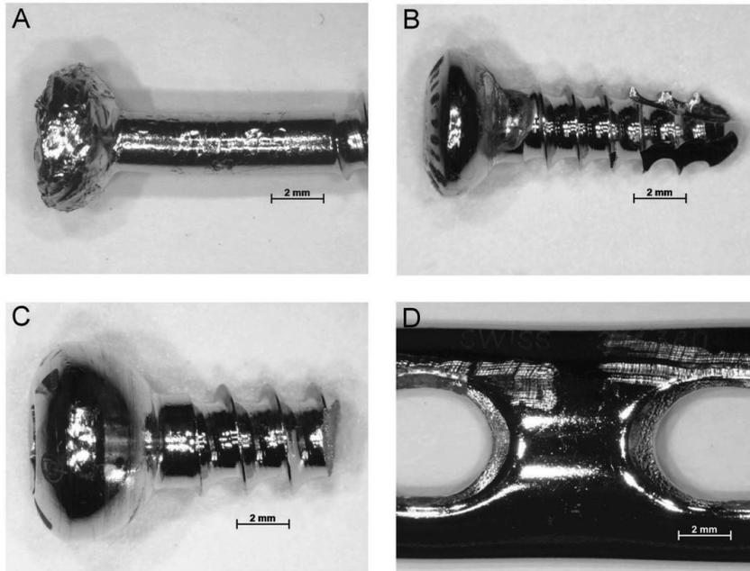
**Figure 3.4:** Stainless steel fracture fixation screws retrieved from patients indicating various defects on screws. A) Defects caused by removal tools. B) Tissue residue and deformation inducing different types of corrosion. C) Screw which was fractured during removal and D) Fixation plate showing *e.g.* marks of deformation.
