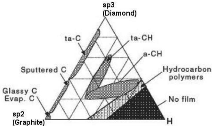
**Figure 4.2:** Phase diagram for various DLC films with respect to their  $sp^3$  and  $sp^2$  and hydrogen contents. (Modified from [134].)
