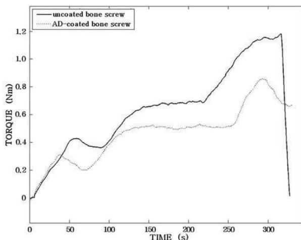
**Figure 7.1:** Insertion torque for two bone screws of diameter 2.7 mm, one with and one without coating. This test was applied to bovine femoral bone, which is significantly harder than human bone.
