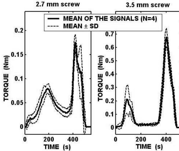
**Figure 7.3:** Mean insertion torque ( $\pm$  SD,  $N = 4$ ) for screws of diameter 2.7mm (left) and screws of diameter 3.5 mm (right). Note the different scales in the y-axis.
