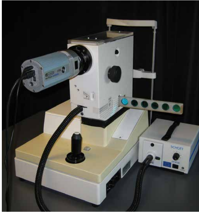
Figure 3.11: The spectral fundus camera system used in Papers I and II.
