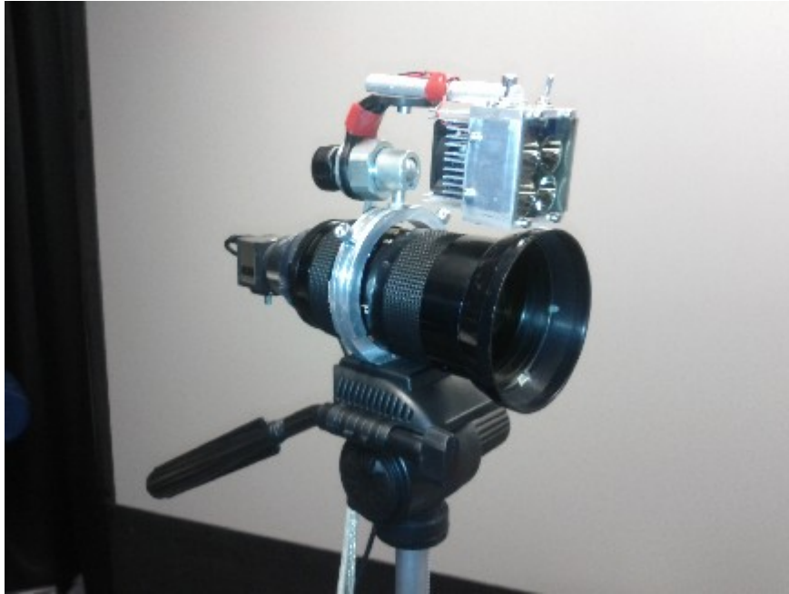
Figure 9: The current version of the hemodynamic imaging system, showing the camera and objective with attached illuminator supported on a tripod.
