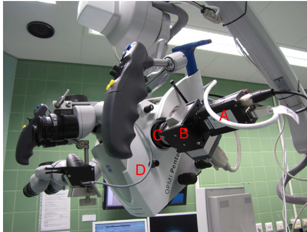
Figure 6.8: The spectral imaging system connected to Zeiss OPMI Pentero neurosurgery microscope. A is the camera, B is the LCTF component, C is optics and D is the microscope.
