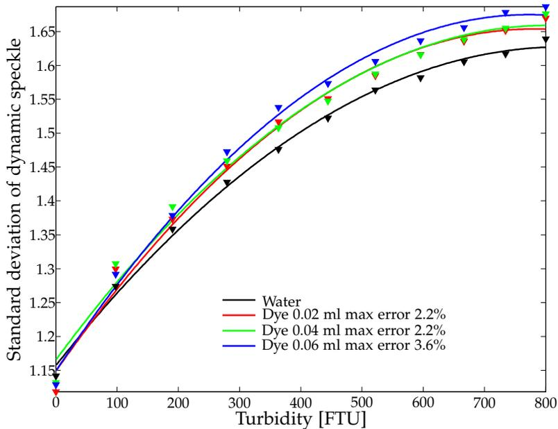
Figure 3.7: Standard deviation of dynamic speckle as a function of turbidity for clear and colored samples.
