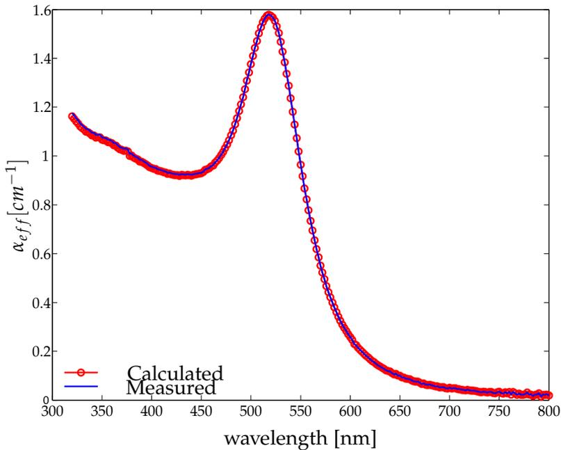
Figure 3.3: Measured and calculated effective absorption spectrum of non-diluted gold colloid.
