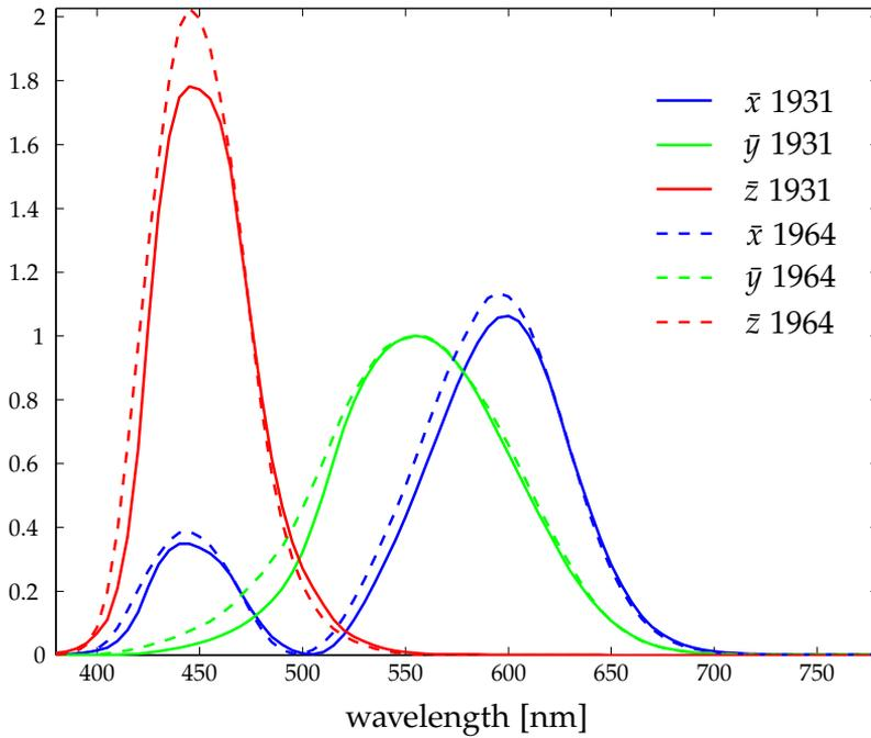
Figure 2.7: Colour-matching functions  $\bar{x}$ ,  $\bar{y}$  and  $\bar{z}$  of CIE 1931 and CIE 1964 observers [58].
