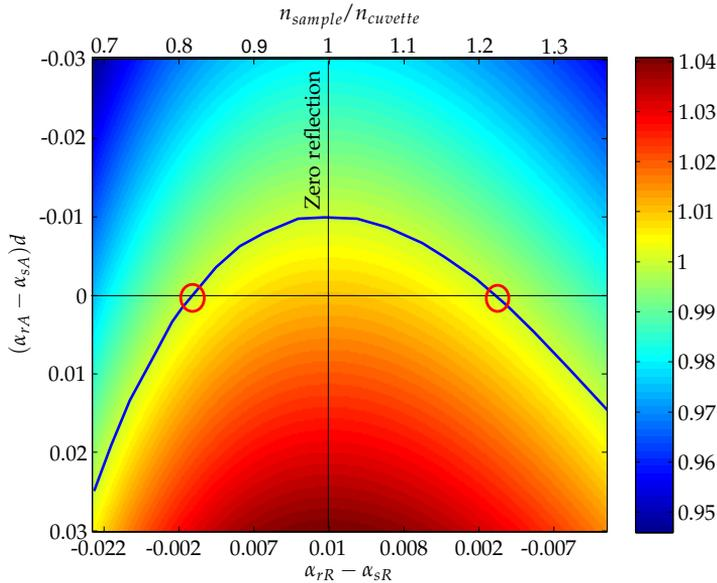
Figure 3.2: Measured and calculated refractive index ratio as a function of the measured absorbance difference between the sample and the reference. The y-axis is the absorbance difference due to the real absorption and the x-axis is the absorbance difference due to the surface reflections. In the x-axis on top of the figure is the refractive index ratio of the sample and cuvette.
