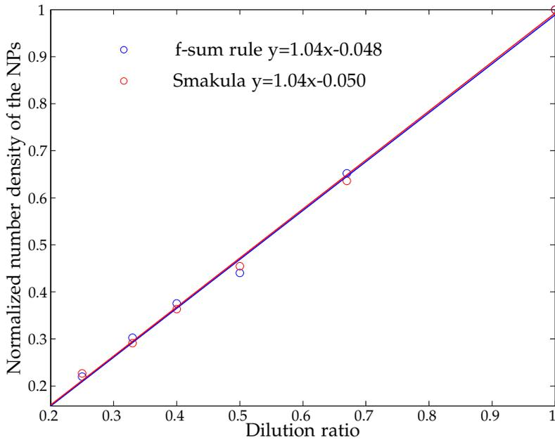
Figure 3.6: Normalized number density of NPs calculated with  $f$ -sum rule and Smakulas formula. Error is estimated to 5 % due to inaccuracy in dilution.
