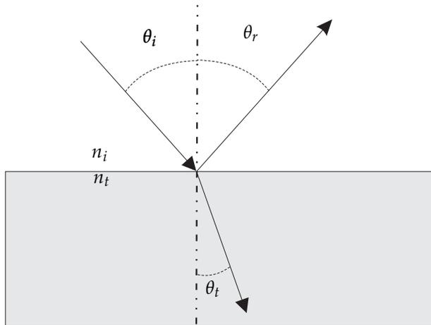
Figure 2.5: Reflection and refraction of a light beam at the interface of two different materials.
