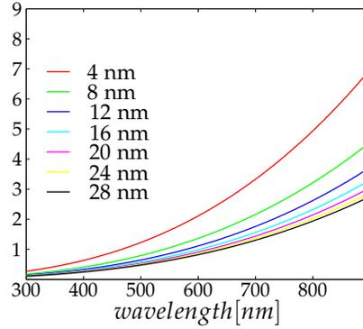
Figure 2.4: The free electron contribution to the  $Im\{\epsilon_r\}$  of gold with different particle radius.
