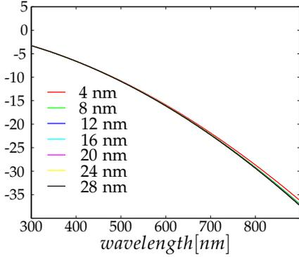
Figure 2.3: The free electron contribution to the  $Re\{\epsilon_r\}$  of gold with different particle radius.
