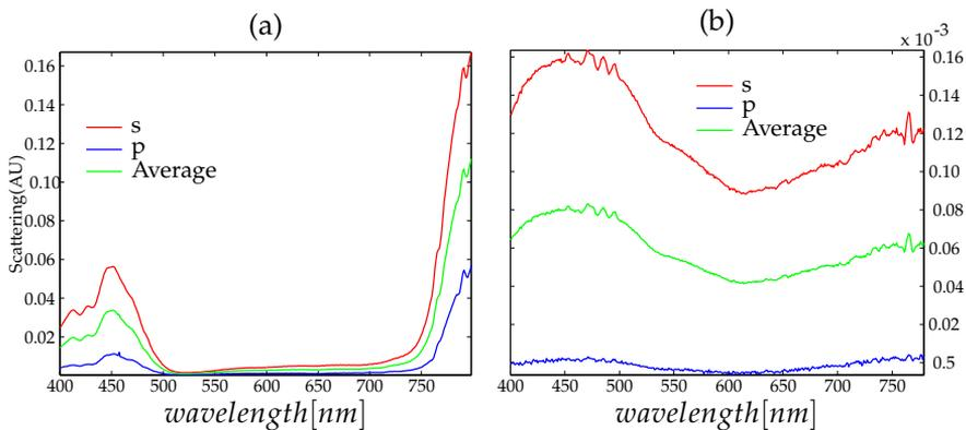
Figure 3.1: The spectra of scattered light of s- and p-polarized and average of s- and p-polarized light from (a)cyan and (b)black ink sample.
