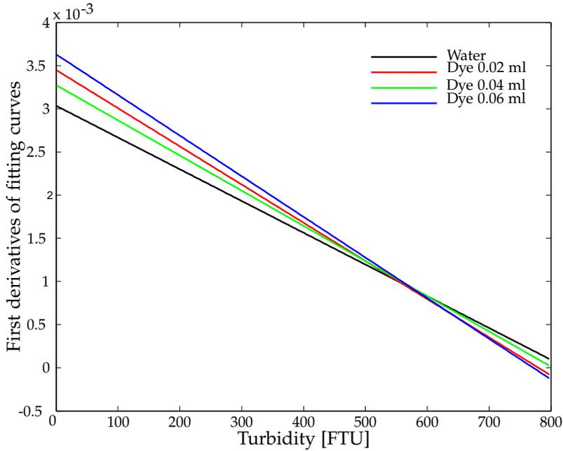
Figure 3.8: The first derivatives of the fitting functions of the measured standard deviation of the dynamic speckle from clear and colored samples.
