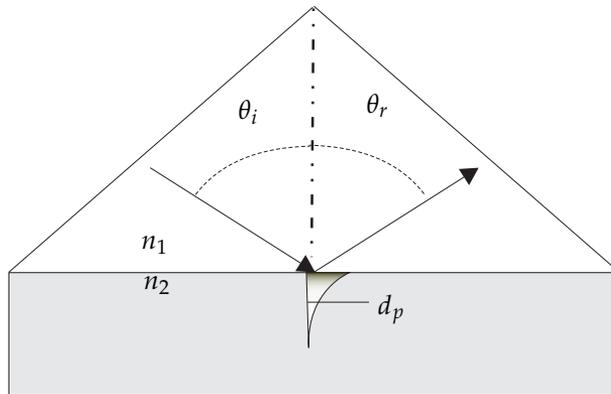
Figure 2.6: Total internal reflection and amplitude of evanescent wave
