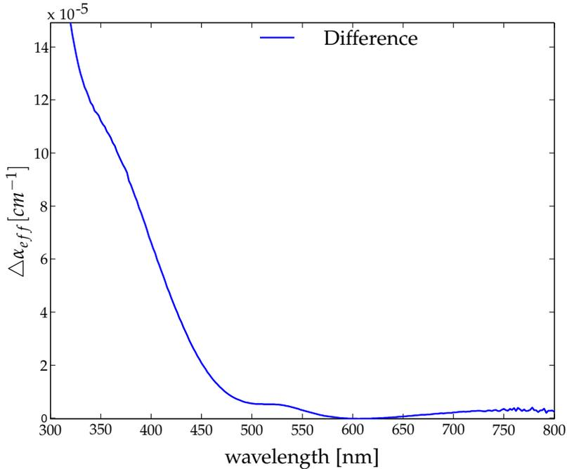
Figure 3.4: Difference of the measured and the calculated effective absorption spectrum of 100 % gold colloid.
