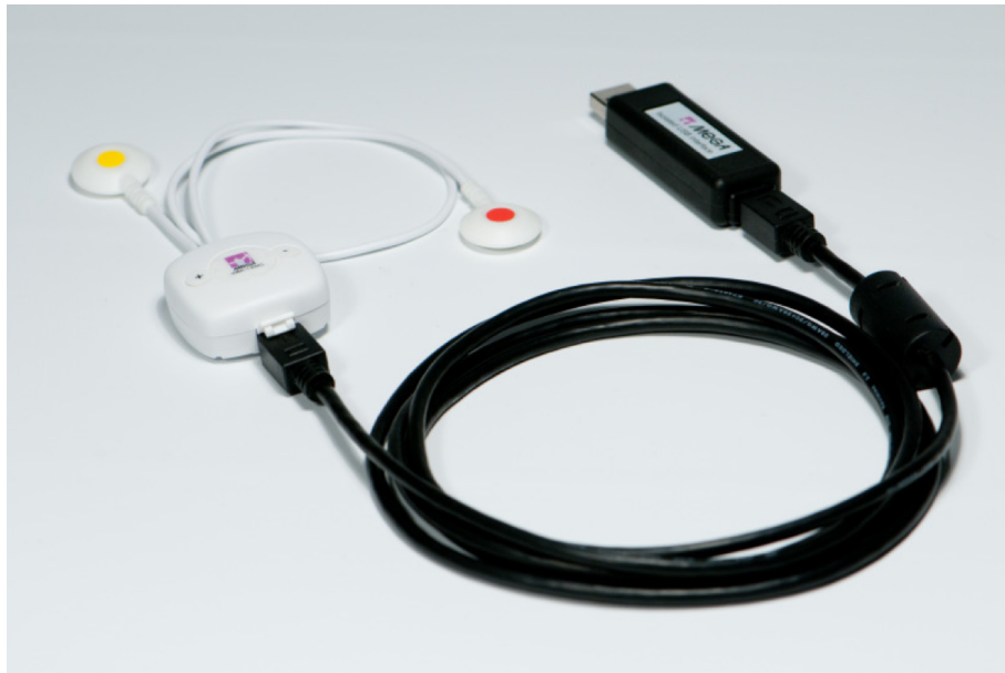
Figure 5.1: The eMotion HRV measurement system, containing the HRV sensor, the USB interface and the USB cable.
