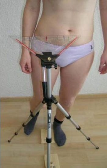
Figure 11. The sideways sway of the belly button was measured with a lineal which was fixed on a tripod.
