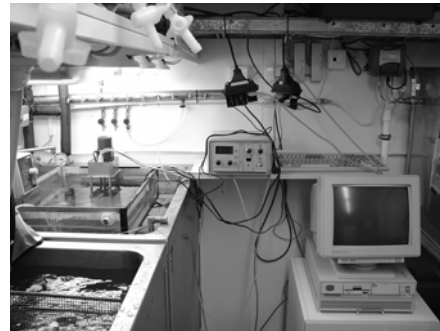
Figure 7. The computer-controlled three-chamber intermittent-flow respirometer (Cyclobios®, Innsbruck) that was used to measure the oxygen consumption of the Arctic charr.
