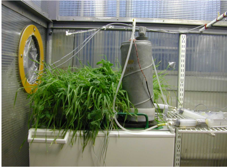
Figure 3. Nine mesocosms placed in the refrigeration unit in the greenhouse. A measurement chamber is placed on top of the mesocosms during the gas flux measurements.
