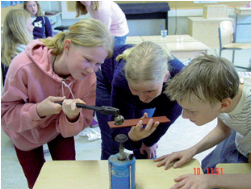
Figure 7. Students heat the metal ball and try to let it pass the hole in the plate. It gets stuck. After some time it falls through. When they try to let the ball pass once more (without heating it) it gets stuck again. Why?
